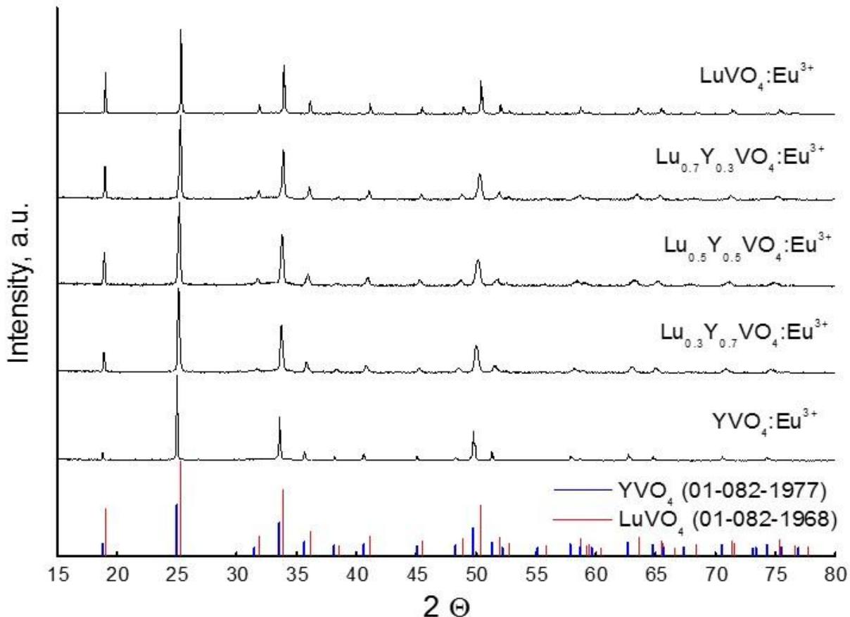
XRD patterns of the  $\text{Lu}_x\text{Y}_{1-x}\text{VO}_4:\text{Eu}^{3+}$  after 1000 °C, 1000 °C, 2 hours, air.
